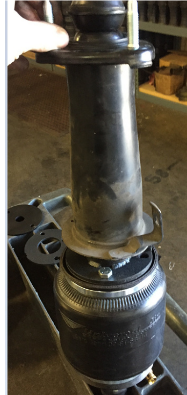
23. Slide oem upper strut mount over bag/strut assembly and re-install top bushing/washer/retaining nut
