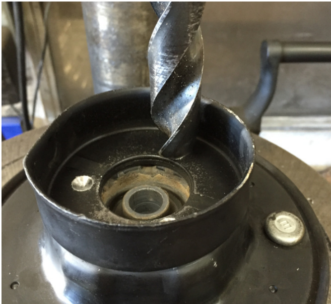
5. Drill Spot welds on upper bump stop cup to strut mount.
