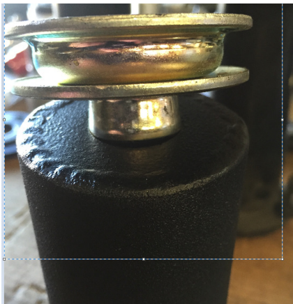
18. Place it into the upper bag bracket with the bump stop nipple facing the mount
