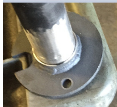
12. If your strut is VERY tight, some persuasion while supporting the bracket will help drive the strut into the mount.
