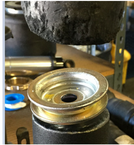
19. Drive in the washer into the mount
