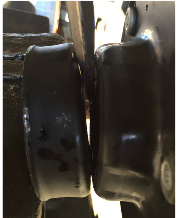
7. Wedge the two pieces apart to finish breaking the welds
