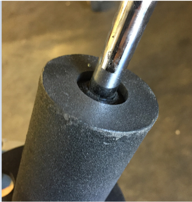
13. Looking from the top, you should see the shock fully seated upto the bottom of the mount.
