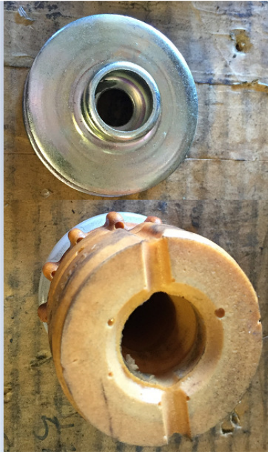
17. After stripping the rear strut bare, take the bump stop and remove the metal washer.
