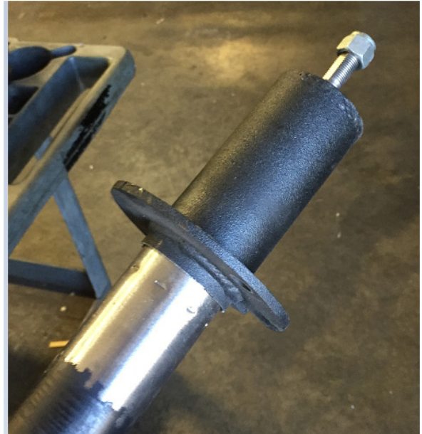
11. Assemble strut and lower bag bracket
