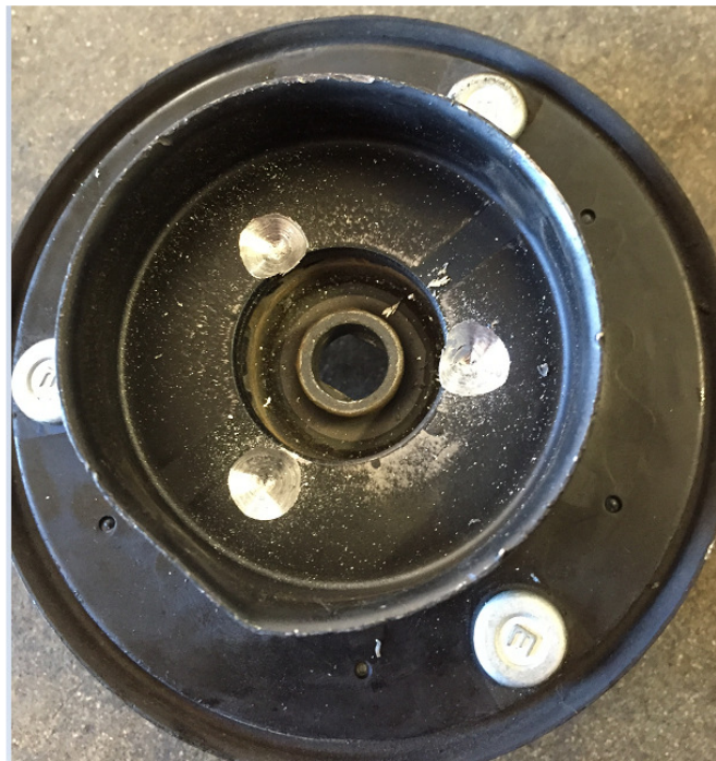
6. Not trying to drill through into the strut mount, just through most of the weld.
