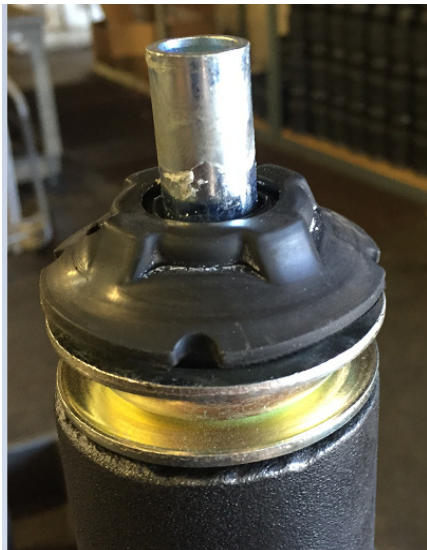
22. Place OEM bushing on top of washer
