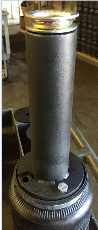
21. Assemble mount on top of bag and plate on bottom of bag with leak tested 90 degree fitting installed
