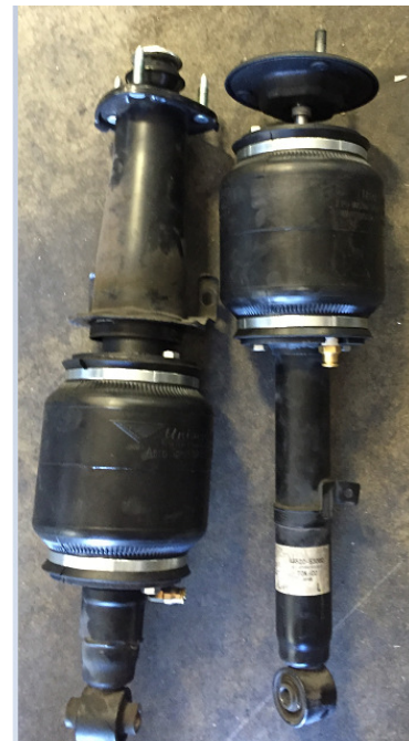
23. Slide oem upper strut mount over bag/strut assembly and re-install top bushing/washer/retaining nut
