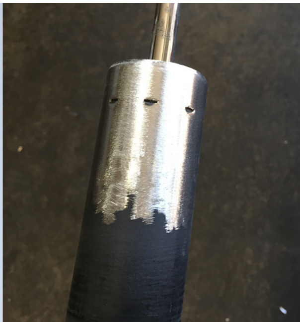
10. Some Struts are large and it's a VERY tight fit into the mount. Light sanding on the end of the strut will make assembly a lot easier.
