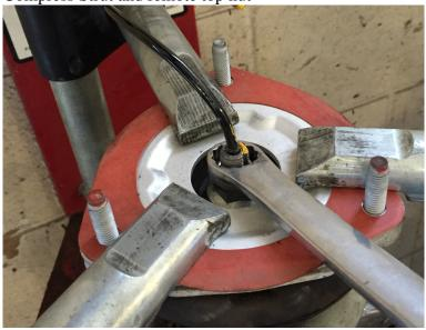
2. Release spring tension and remove top strut mount, coil spring and isolators
