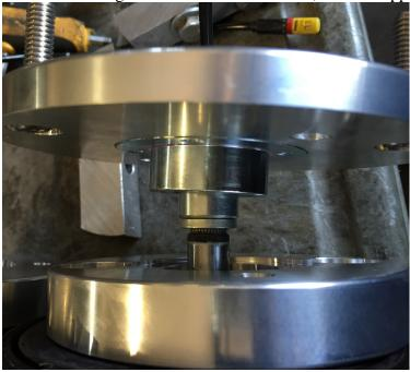
10. Temporarily remove the bag bolts holding the upper mount to the bag. Slide mount over upper strut mount to gain access to clamp shock shaft with a soft material to not damage shock shaft.
